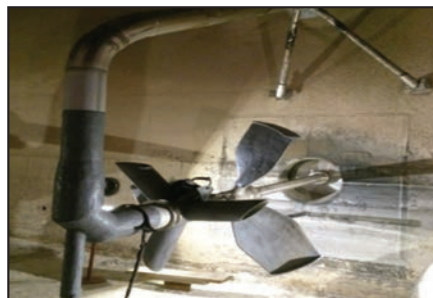
Mixer and lance with the applied ARC 855 and ARC BX2 coatings.
