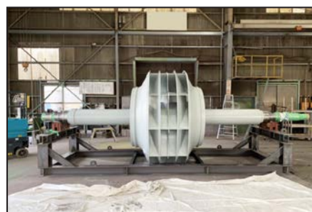
ID Fan in paint shop.
