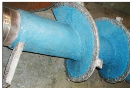
ARC MX1 applied and tips welded.
