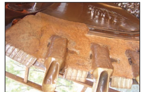
After 20 months only 5 kg of ARC BX1 was needed for repair.
